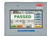
Generic HMI viewers with dedicated software to manage TM3 test modules
